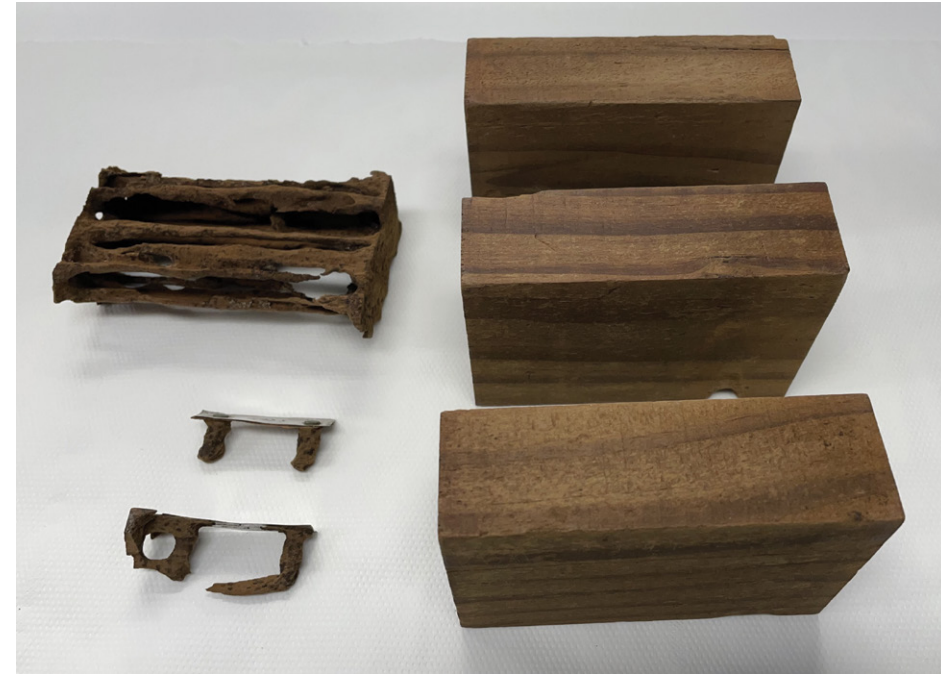
Comparative performance of Vulcan Radiata 230°C untreated (left) vs LOSP Azole and permethrin treated (right), when exposed to Coptotermes acinaciformis termites in AWPC H3 field test, Queensland.
