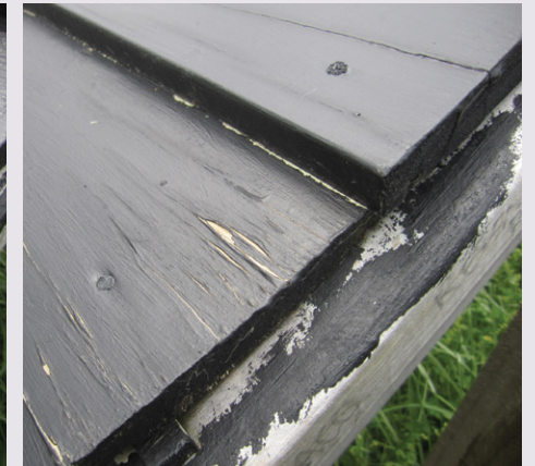
MCA Treated KD Radiata Pine, 3 years exposure.
